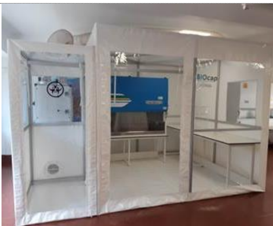
BIOcap prototype in positive pressure (protection of the interior from the surroundings)
